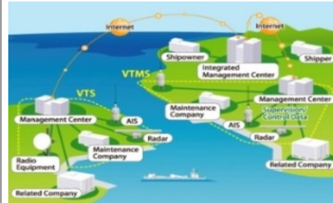
Image of VTS/VTMS System ※VTS: Vessel Traffic Services, VTMS: Vessel Traffic Management System (Both of them are control system of marine traffic)
